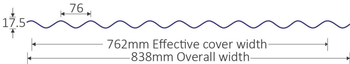
The Corrugated profile virtually eliminates oil canning and the sheeting can be factory cranked, curved and bull nosed to various radii depending on customer's requirements. The overall width of a Corrugated sheet is 838 mm.
